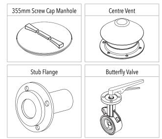
$^{\rm 1}$  Standard sizing of Butterfly Valve and Stub Flange 3", 4" and 6", other sizes available on request
